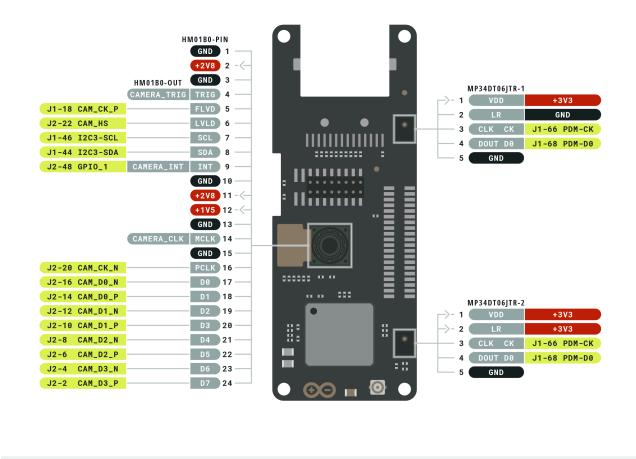
The pinout for the Portenta Vision Shield LoRa® is shown in the figure below.
